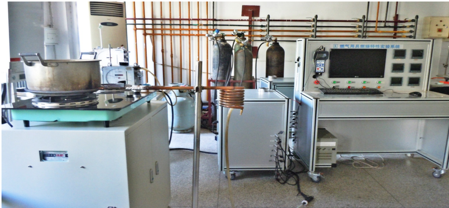
Figure.2 Schematic diagram of gas combustion characteristic and gas appliance adaptability experiment system (GCTS)
